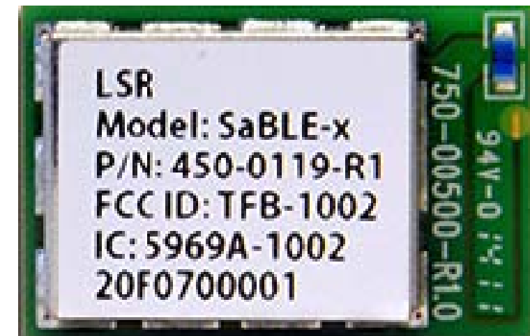
Off-the-shelf wireless platforms such as the SaBLE-x Bluetooth Smart module can be leveraged in connected systems to circumvent the costs associated with Intentional Radiation testing. Source: nuvation.com
